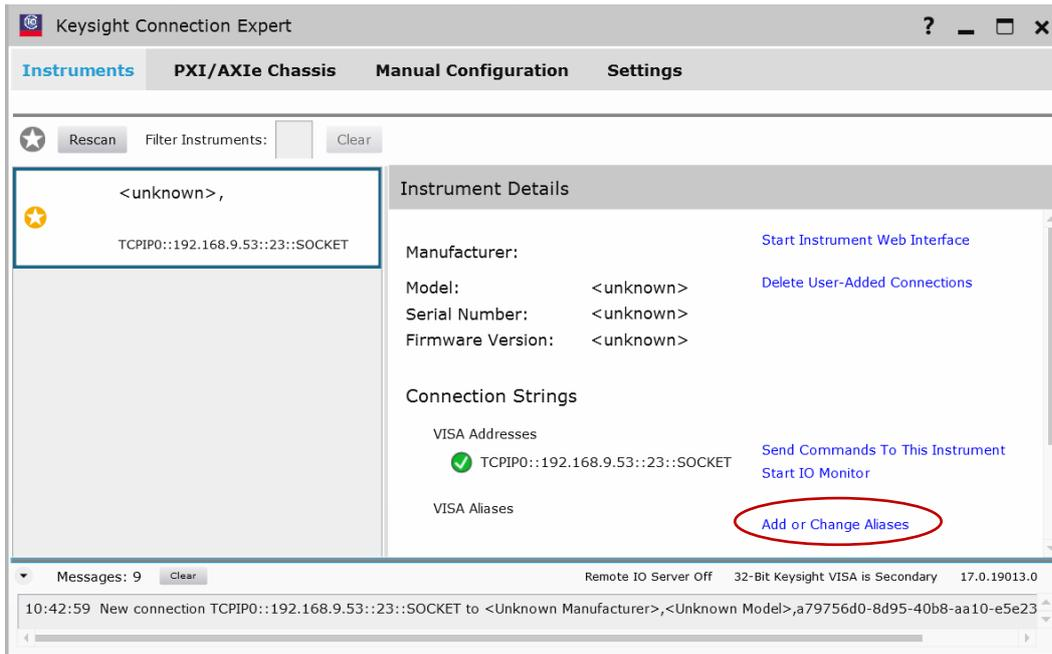
Fig iii - Connection Expert home screen summarising the new LAN instrument (Add or Change Aliases is highlighted)
