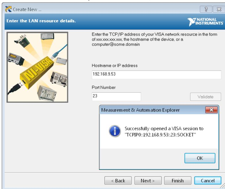
Fig v - Successfully testing the LAN configuration
